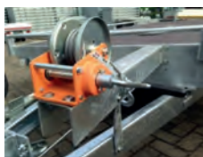
Fig. Option: Winch + cable + brace
